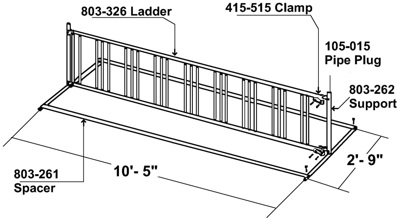
Main Frame, legs and spacers are 1 5/8" O.D. hot galvanized welded pipe with 3/4" O.D. hot galvanized ladder rungs. Spacing between tire posts is 3" center-to-center for small gap, 8 1/2" center-to-center for large gap.
